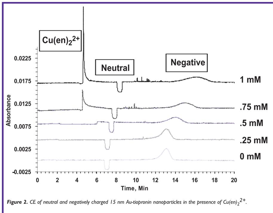
Figure 2. CE of neutral and negatively charged 15 nm Au-tiopronin nanoparticles in the presence of  $\text{Cu}(\text{en})_2^{2+}$ .
