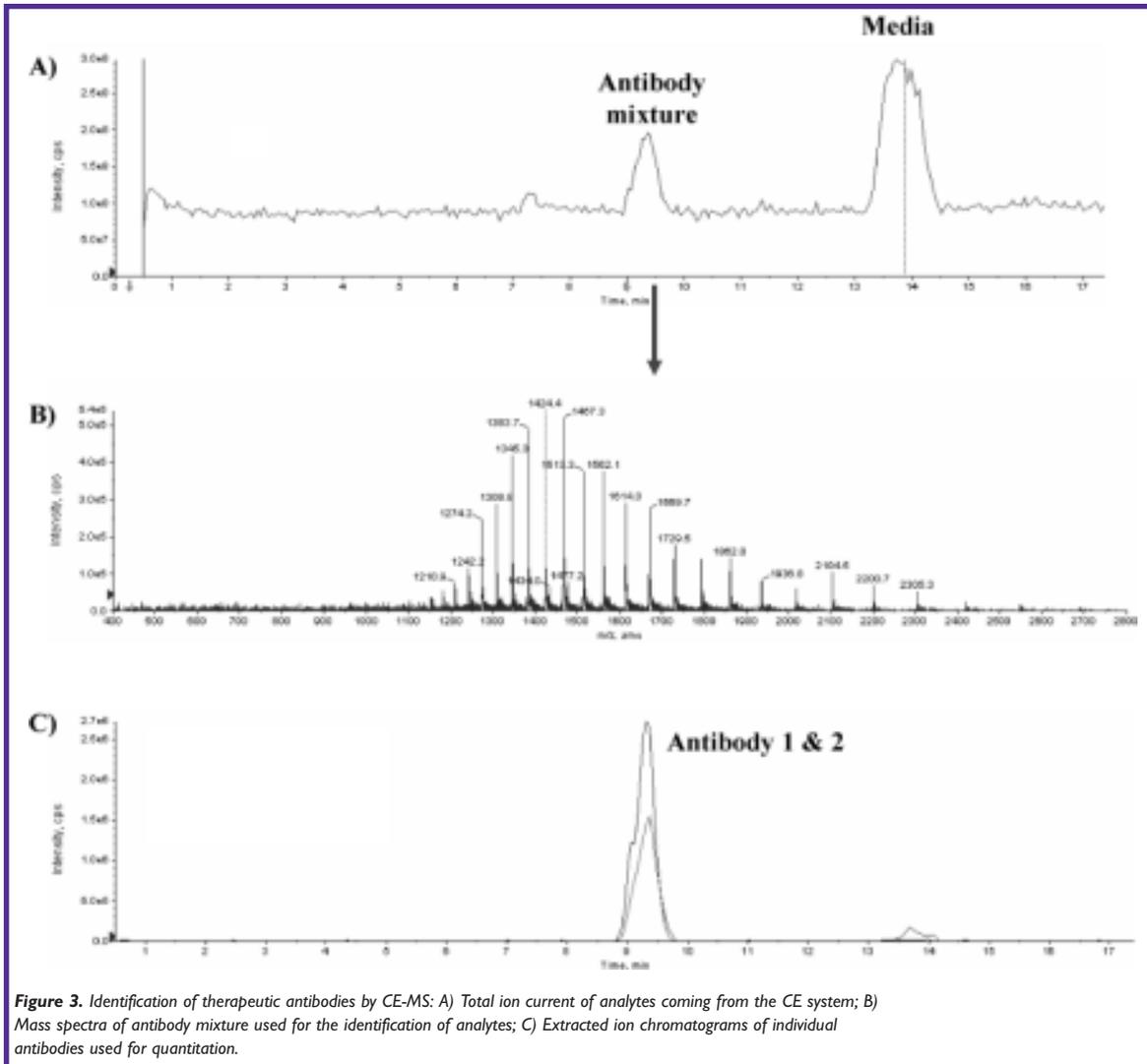
Figure 3. Identification of therapeutic antibodies by CE-MS: A) Total ion current of analytes coming from the CE system; B) Mass spectra of antibody mixture used for the identification of analytes; C) Extracted ion chromatograms of individual antibodies used for quantitation.
