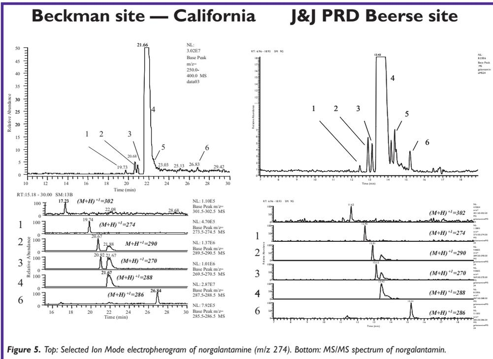
**Figure 5.** Top: Selected Ion Mode electropherogram of norgalantamine ( $m/z$  274). Bottom: MS/MS spectrum of norgalantamine.
