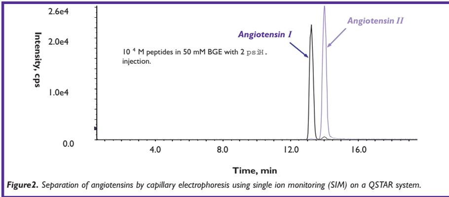
Figure 2. Separation of angiotensins by capillary electrophoresis using single ion monitoring (SIM) on a QSTAR system.
