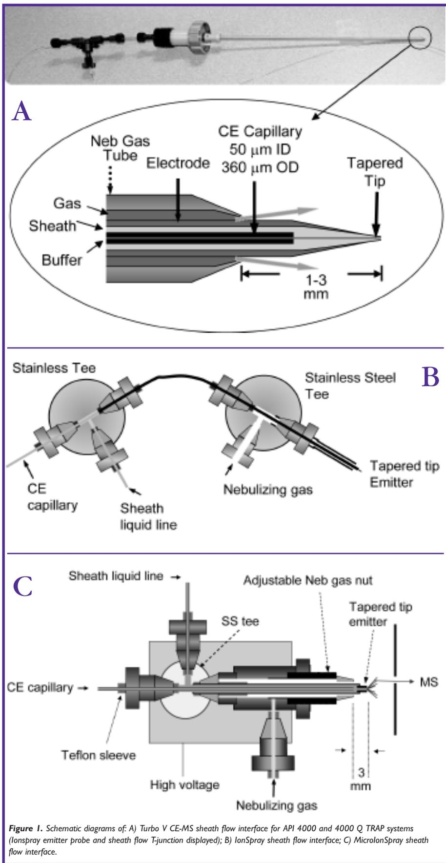
**Figure 1.** Schematic diagrams of: A) Turbo V CE-MS sheath flow interface for API 4000 and 4000 Q TRAP systems (IonSpray emitter probe and sheath flow T-junction displayed); B) IonSpray sheath flow interface; C) MicrolonSpray sheath flow interface.
