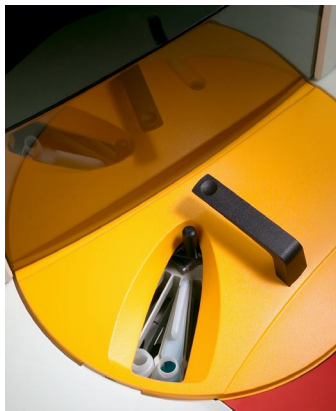
Figure 1-5a: Reagent vials and the 35-position reagent disk in the Konelab 20 and 20XT
