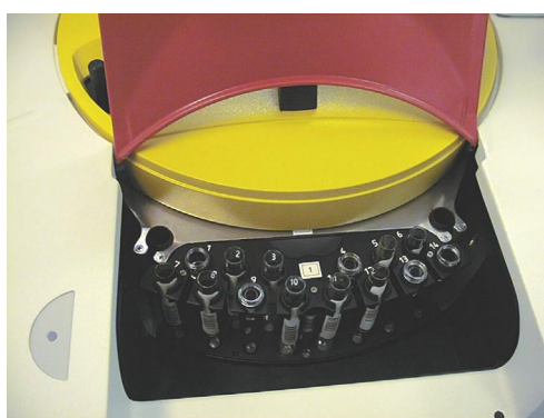
Figure 2-5b: In Konelab 20XT and 20 calibrator, control and antigen excess samples are loaded into segments as normal samples. ISE prime sample is always inserted into the sixth STAT position.
