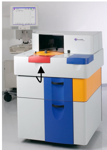
Figure 8-3: When detaching the sample disk in Konelab 20XT and 20, open the whole dispensing cover. There is a bearing rod to keep the cover up.
