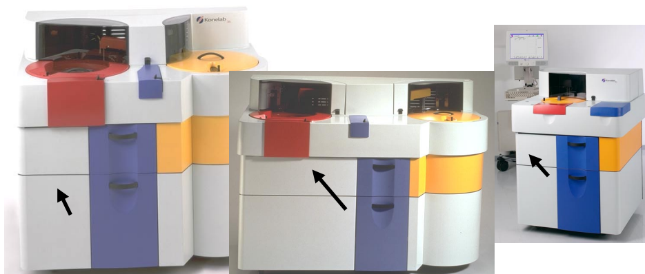
Figure 6-1: Location of the lamp housing is behind the front panel
