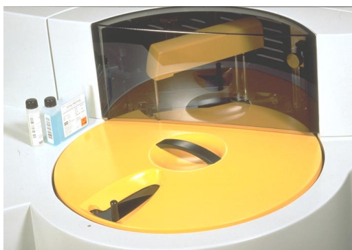
Figure 1-5b: Reagent vials and the 45-position reagent disk in the Konelab 30 and 60
