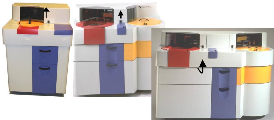
Figure 6-7: When replacing mixing paddles in Konelab 60, lift the whole of the top cover and support with the bearing rod. In Konelab 30 and 20XT is only necessary to open the upper cover.
