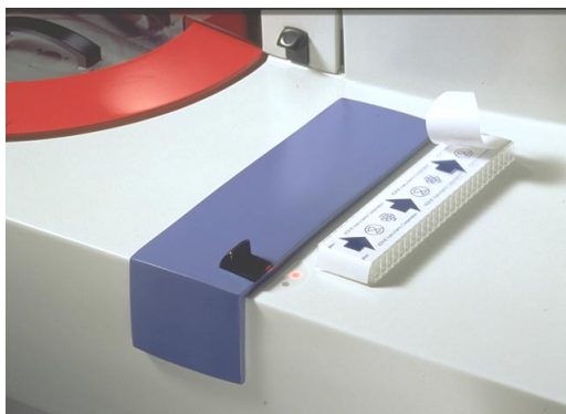
Figure 2-4a: The cuvette loader and a cuvette packet in Konelab 60/30.
