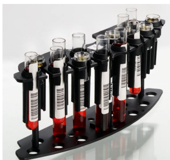
Figure 1-2: A sample segment
