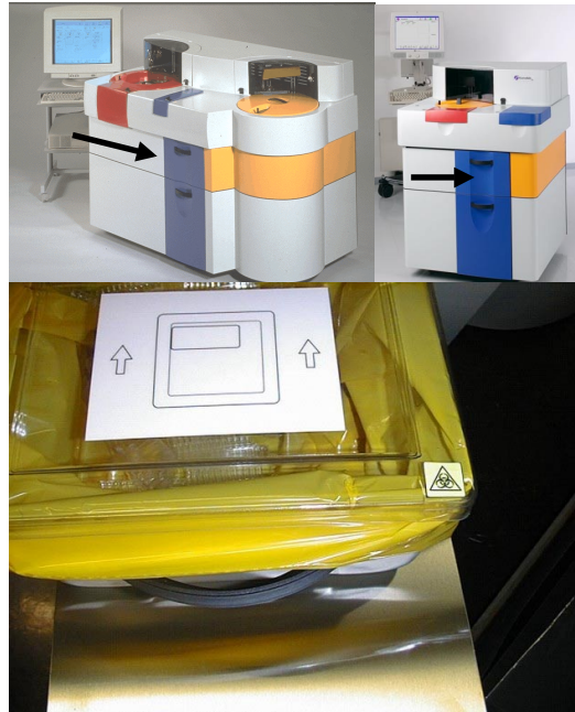
Figure 2-2: The cuvette waste compartment is located in the upper drawer of the analyser stand. Place the cover of cuvette waste box so that arrows show away from you.
