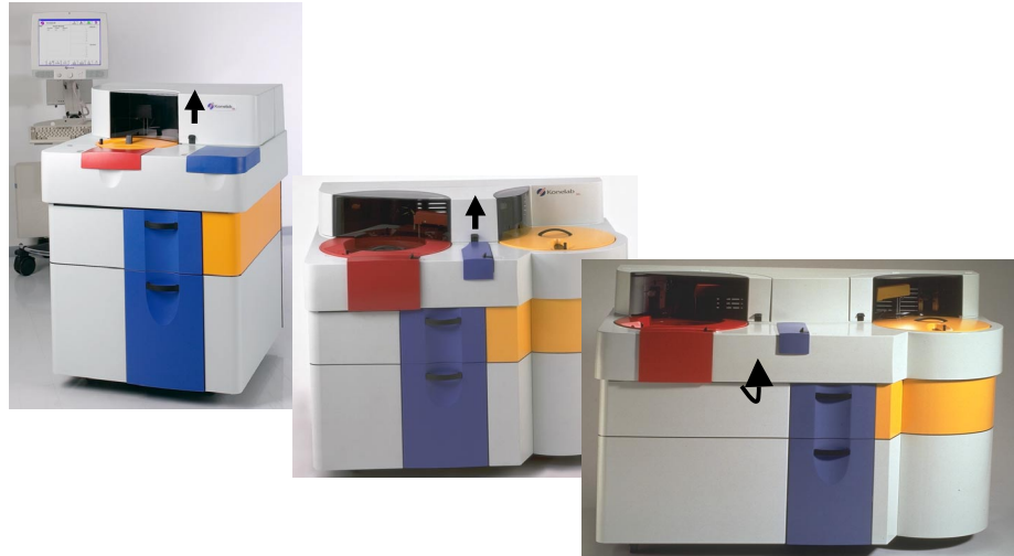
Figure 8-2: When removing cuvettes from the incubator in Konelab 60, open the whole top cover and support it with a bearing rod. In Konelab 30, 20XT and 20 is only necessary to open the upper cover.
