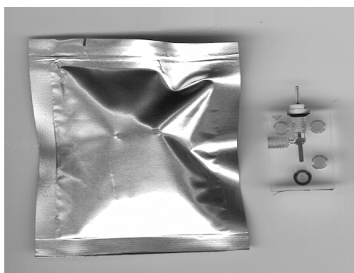
Figure 9-8: Foil bag containing an electrode and the electrode
