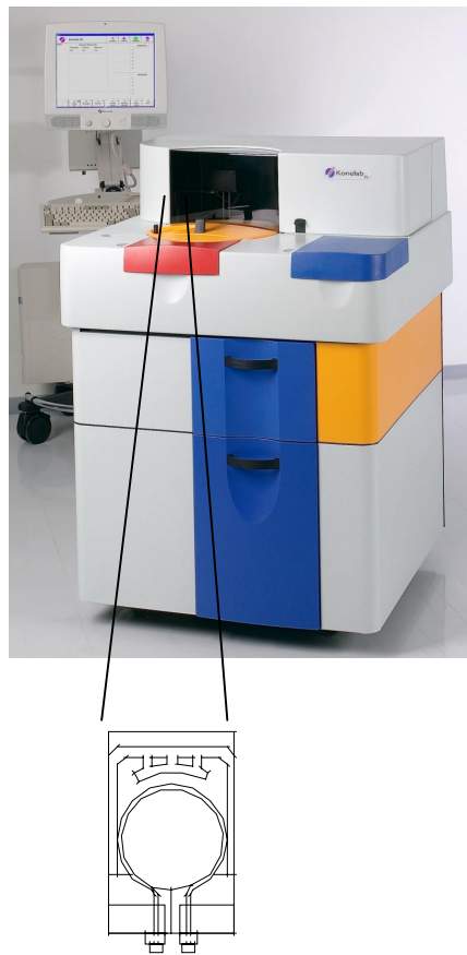
Figure 6-8b: The place of the ISE washing pump in Konelab 20i
