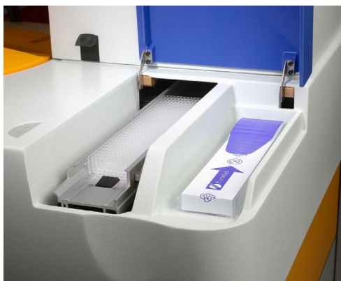
Figure 2-4b: The cuvette loader and a cuvette packet in Konelab 20XT/ 20.
